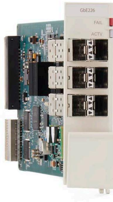
Figure 2. The new Tellabs 10 Gigabit Ethernet 226 (GbE226)
